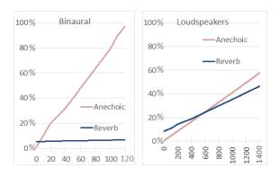
Figure 1. Performance of the spatialisers depending on the number of sources. The horizontal axis shows number of sources and the vertical axis shows percent of total buffer time (~11.61 ms). Left: binaural spatialiser. Right: loudspeakers-based spatialiser.
