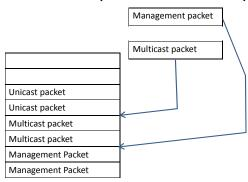
Figure 1. Insertion of the packets in the queue using priority criteria
